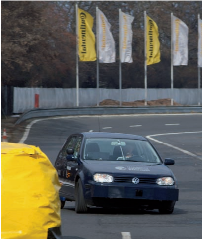
Figure 6: Test vehicle and crash safe obstacle while performing an emergency steering maneuver
