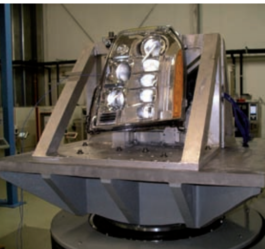
Figure 3: Vibration test on the test rig for safeguarding the strength simulations
