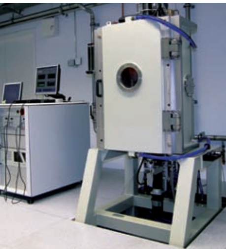
Kistler's facility for growing „PiezoStar“ crystals from the melt
