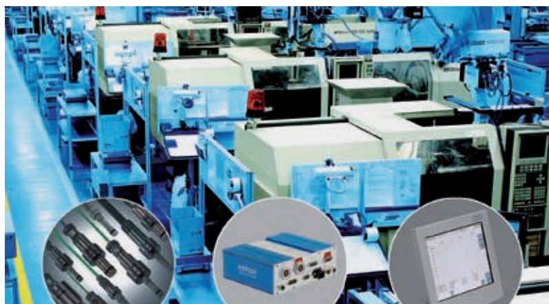
„CoMo Injection“ systems guarantee zero-defect production and process transparency during injection molding
