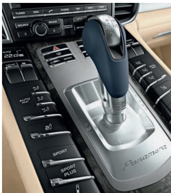
Figure 1: The selector gate of the Porsche double-clutch transmission PDK in the of the Porsche Panamera with selector buttons for the Sport and Sport Plus modes (bottom left)
